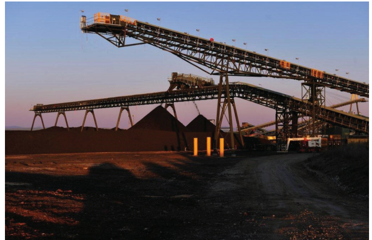
Above: (L) Skyline conveyor with tripper in operation and stockpile conveyor
