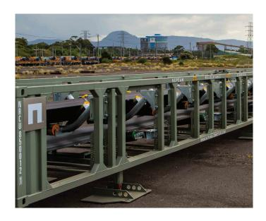
Larger belt widths of up to 1.8m can be accommodated on conveyors without horizontal curves. When you partner with NEPEAN Conveyors you get a complete solution, not just part of the supply. Our innovative design has all the system components you need for a fully operational, relocatable, reusable modular conveyor system, from our foundationless combination drive and loop take up, to our one-piece tail end loading station. We can provide everything you need in one low cost turn key system.
